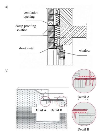
Fig. 2. a) Example of the gap sealing between the aluminium window and doorjamb in three-layer wall by [2]; b) the sample brick lintel in the three-layer wall by [3]
